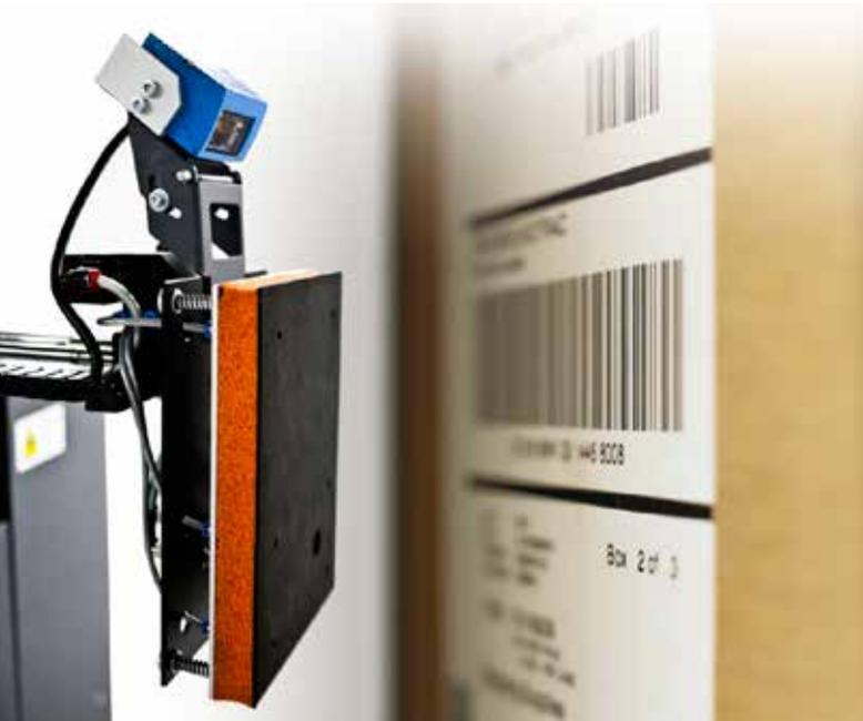
Secondary packaging print and apply labelling is done in real time. In order to achieve optimisation in all production processes, the automation of each phase of the production stage is crucial, as is the solution adopted, and the machinery selected to carry out the task.
